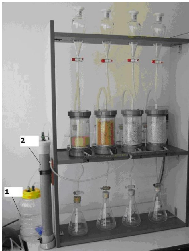
Fig.4.1.1 – Photo of the kinetic test installation, based on the Humidity Cell Test; 1 – Air humidifier; 2 – Air drying column
