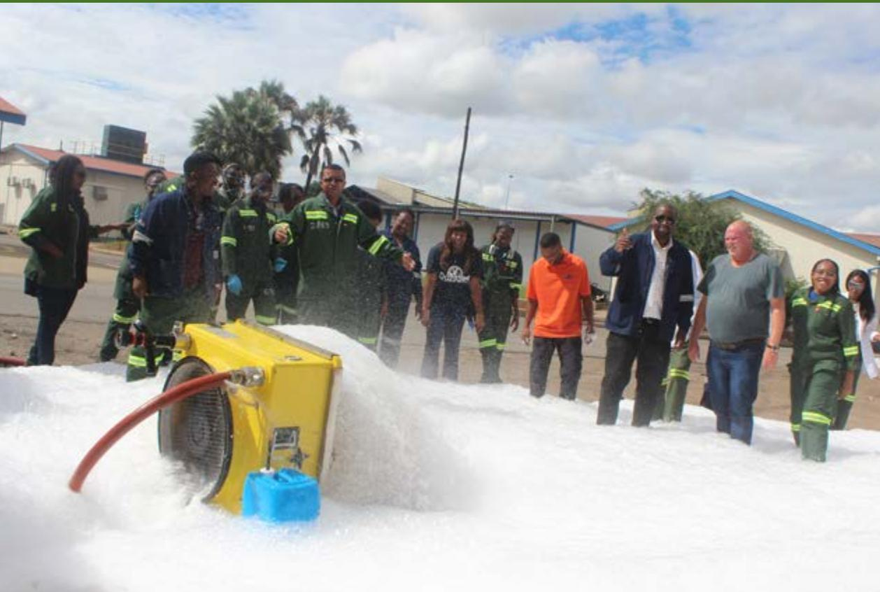
*The Dundee Precious Metals Tsumeb Emergency Response Department showcase the portable foam generator. It is designed to expand foam solution into millions of tiny stable bubbles specially engineered to extinguish chemical fires*
