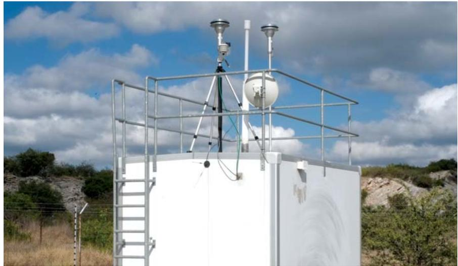
Sulphur dioxide (SO<sub>2</sub>), particulate dust (PM10) and arsenic (As) monitoring station – Tsumeb.
